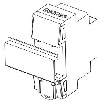
Figure 3: Mounting MINiBOX 0-10V X3 on DIN rail
