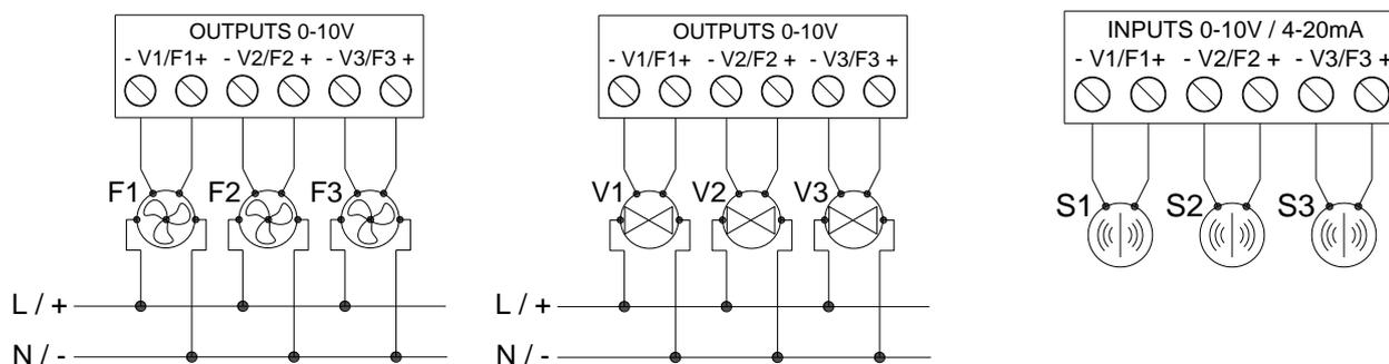
Figure 2: Wiring examples
