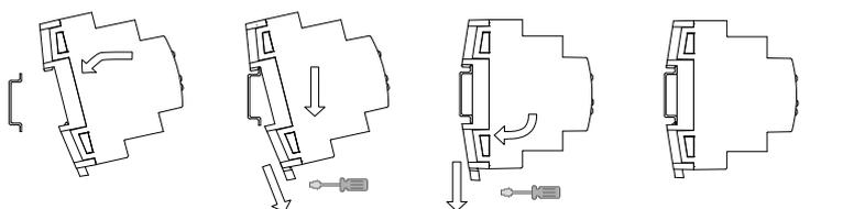
Removing MINiBOX 0-10V X3 from DIN rail:
