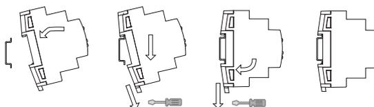
Removing DIMinBOX DX1 from DIN rail:
