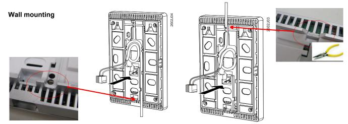
Remove the breakout on the housing before putting the cable into the gaining channel.
