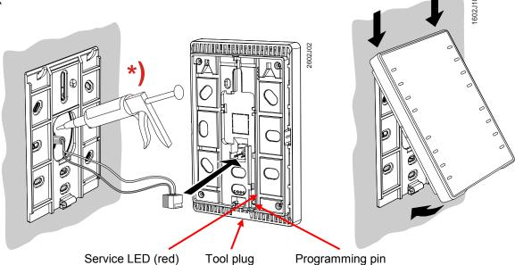
\*) The installing tube must be sealed or cold or warm air may enter the device and cause faulty temperature readings by the internal sensor.
