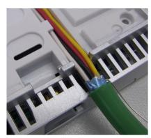
Remove the cable coating, as it will not fit in the gaining channel.
