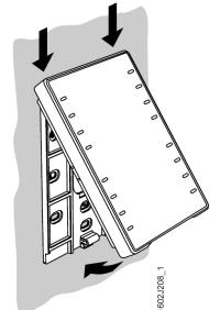
The installing tube must be sealed or cold or warm air may enter the device and cause faulty temperature readings by the internal sensor.
