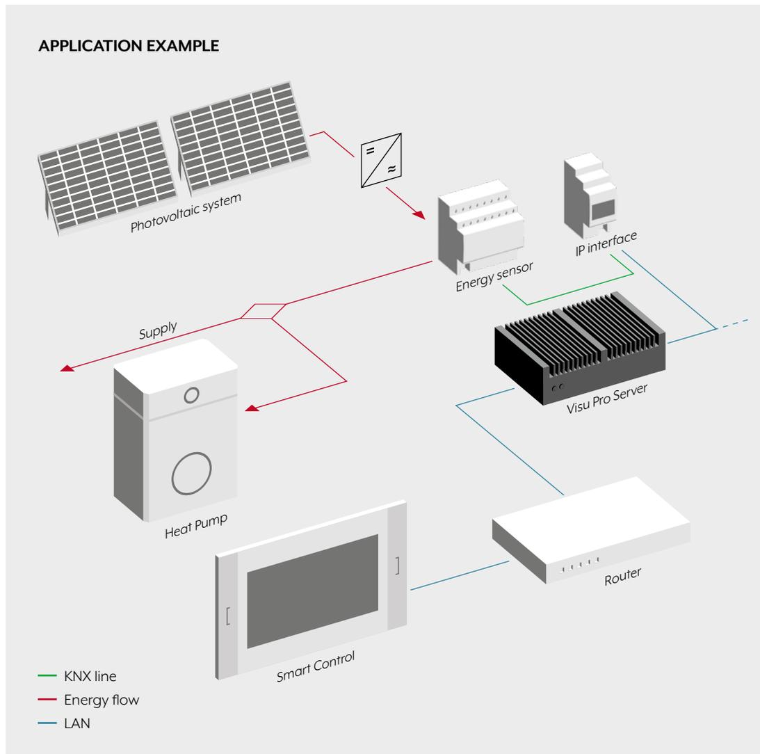
The KNX energy sensor has three channels for connecting to consumers. For each channel, energy amounts, voltage, current and effective and reactive power are measured. Alternatively, it also records three-phase current levels. The sensor cyclically sends the data for evaluation and visualisation to the KNX bus. With the converter measurement function, it can also measure the complete consumption up to 75 ampere – as well as the existing three
