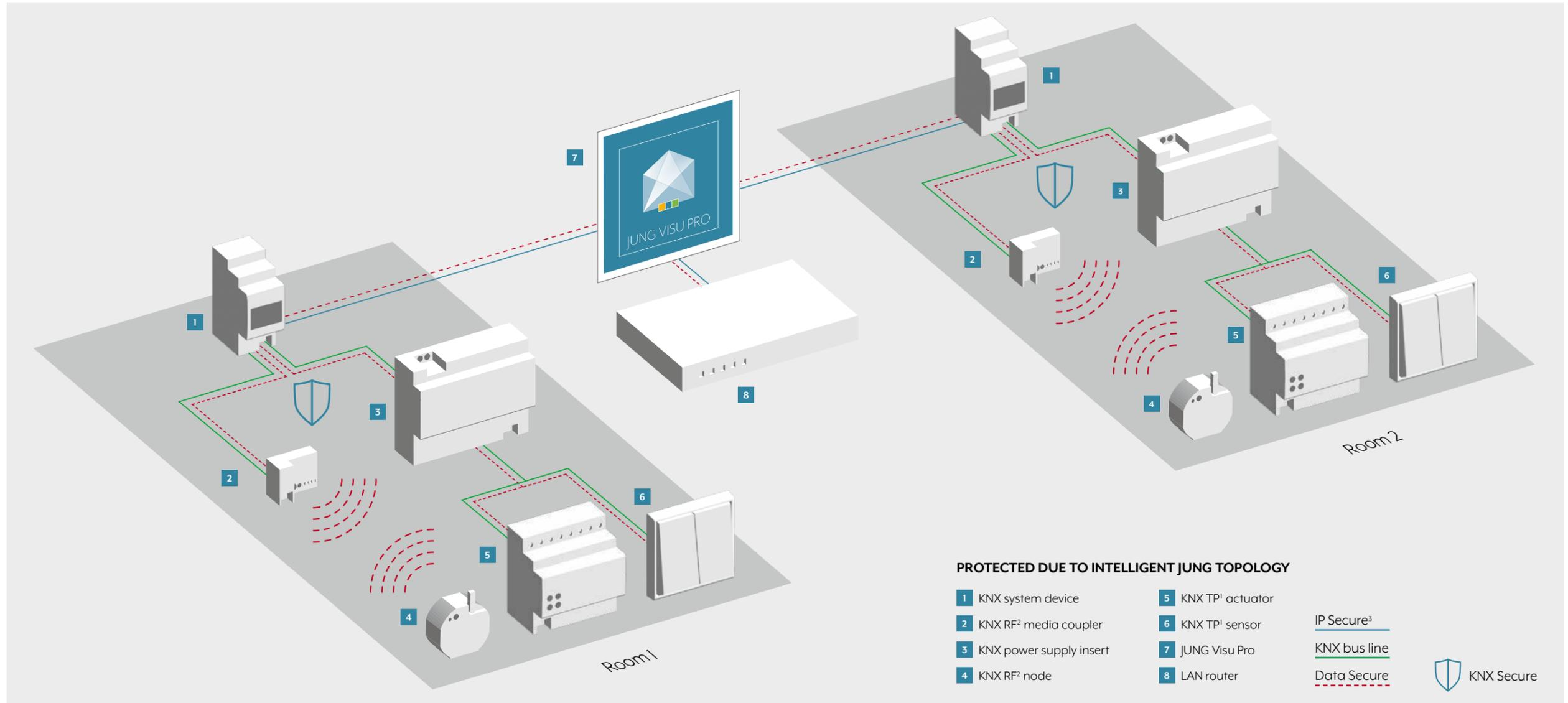
The discussion about data protection also does not stop at a smart building. Because everything you can operate digitally yourself, can theoretically also be controlled by unauthorised third parties. This is where JUNG KNX Secure comes in and provides effective protection thanks to encryption with the AES128 algorithm.
