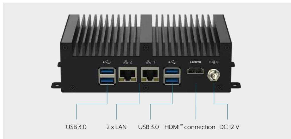
The JUNG Visu Pro Server is the compact solution for controlling building automation in conjunction with the pre-installed Visu Pro software. Ideal for applications in challenging private construction.
