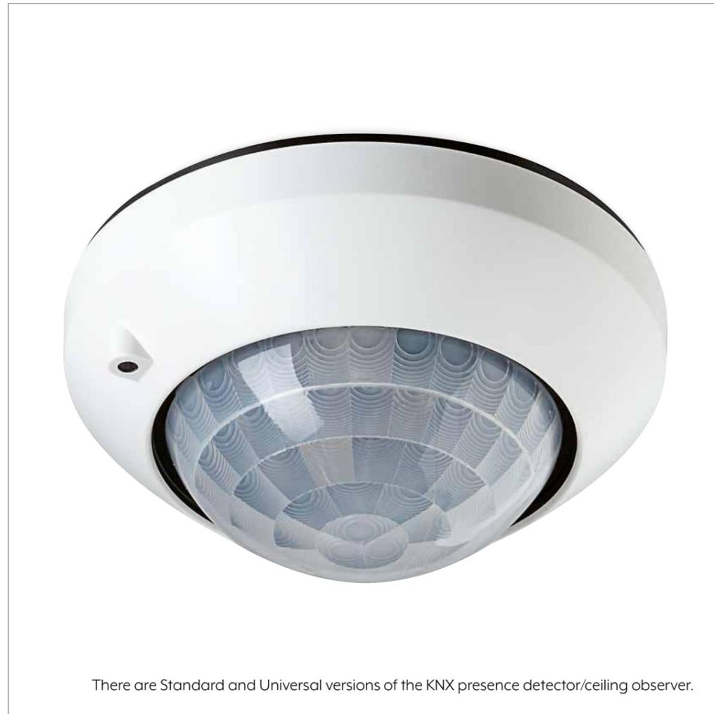
This presence detector/ceiling observer is reliable. Even when great height is a problem. When installed at heights of up to 5 m, the unit registers everything that is moving within a diameter of approx. 20 m. The detection angle of 360° can be divided into three sensor segments of 120° each that can be enabled individually.
