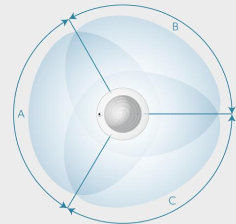
There are Standard and Universal versions of the presence detector/ceiling observer. In addition to presence-dependent constant light regulation, the Universal model also has five function blocks that operate independently of each other and to which the three PIR sensors can be assigned. Each functional block may be configured as desired for the presence detector, ceiling observer, or signalling applications.
