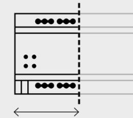
The width of the dimming actuator is only 4 TE. This effectively saves space in the distributor.
