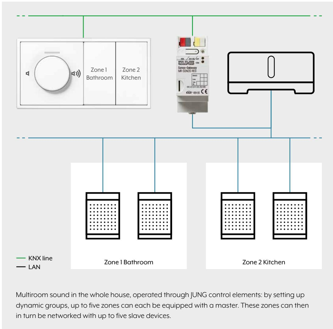
The new JUNG KNX Sonos Gateway connects the intelligent KNX technology with Sonos multiroom sound. Intuitively controlled using KNX sensors or smartphone/tablet in connection with the Smart VisuServer: up to 30 Sonos
