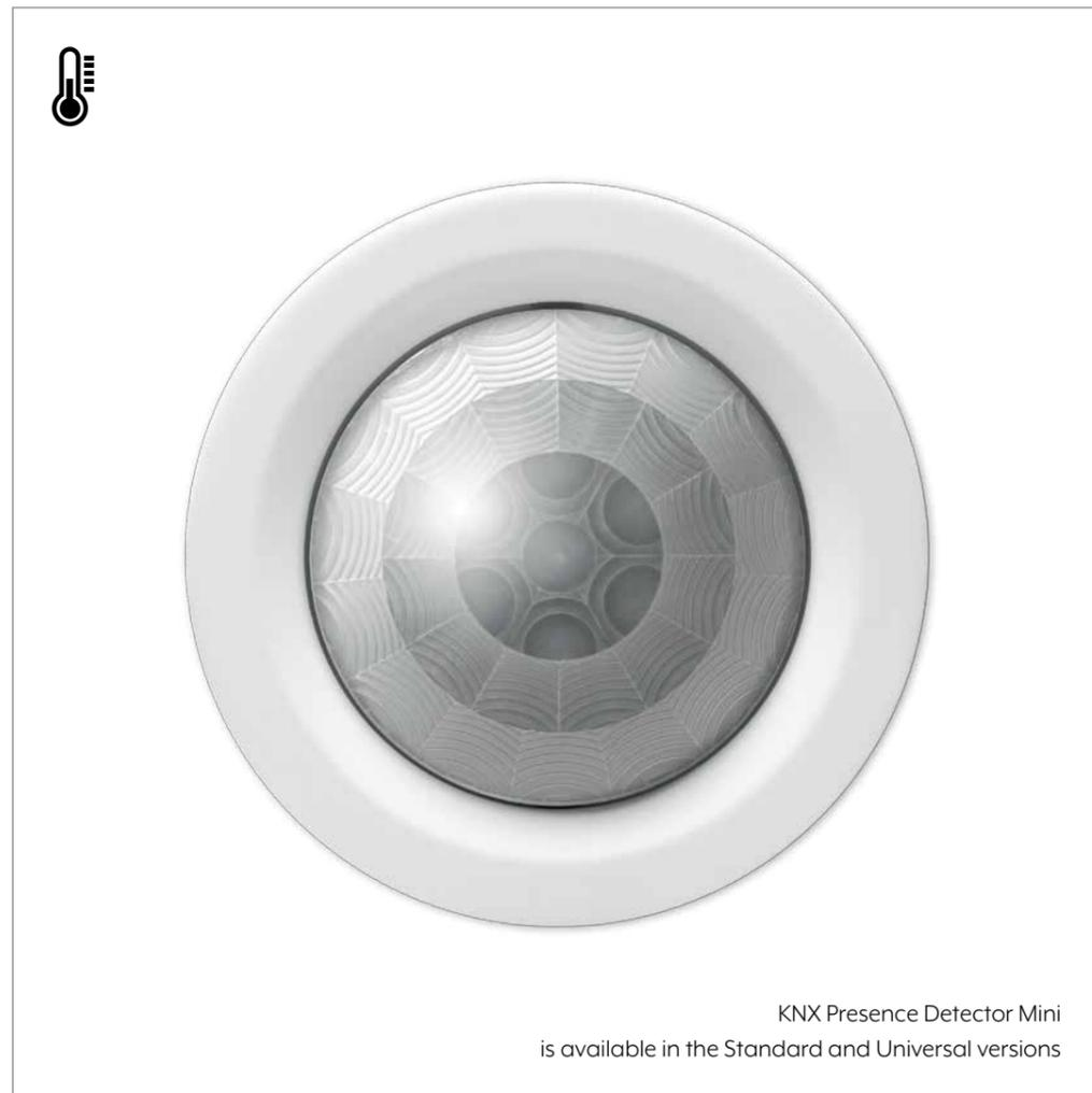
Unobtrusive, compact, precise: the KNX presence detector mini is all of these. It is designed to control lighting systems, room thermostats, and other electrical loads as needed. The striking feature is its compact design with three ceiling mounting options: Depending on the particular room situation, the unit may be installed in a false ceiling, on the surface, or in a commercial flush wall box.
