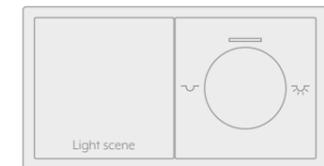
All three binary inputs of the rotary sensor are used here: activate lighting scenes via the connected push-button, dim all connected luminaires together with the rotary sensor and also move the shutters up and down using the blind push-buttons.
