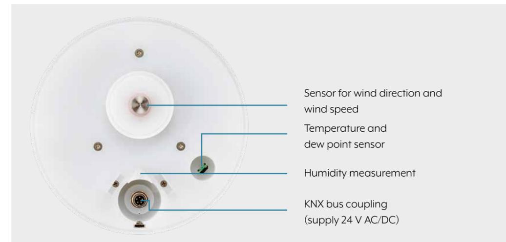
Wind speed, wind direction, brightness – in four directions, twilight, global radiation, precipitation, relative air humidity and air pressure are measured using the integrated sensors. The calculation of further data such as absolute humidity and perceived temperature is also carried out. Operating interdependently with each other, values are also determined in terms of the mugginess curve and comfort characteristic that can then be used to optimise the ventilation control. These features
