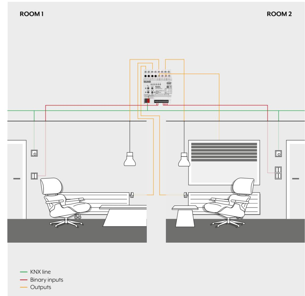
The JUNG KNX Multistation is a real problem solver. The REG housing has only 4 TE and offers a unique combination of six push-button interface, six switch outputs, two integrated room temperature controllers and two inputs for temperature sensors. This allows, for example, a complete office, hotel or hospital room to be equipped with all necessary
