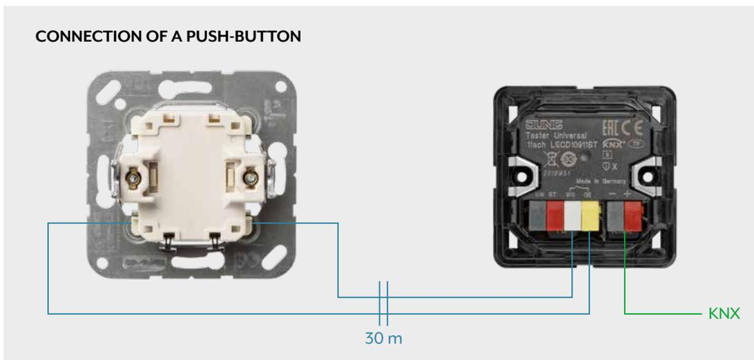
An extension connected to a KNX F 10 push-button sensor Universal can be placed at a distance of up to 30 metre cable length in the process. Thus the JUNG KNX push-buttons F 10 enable a smart and at the same time
