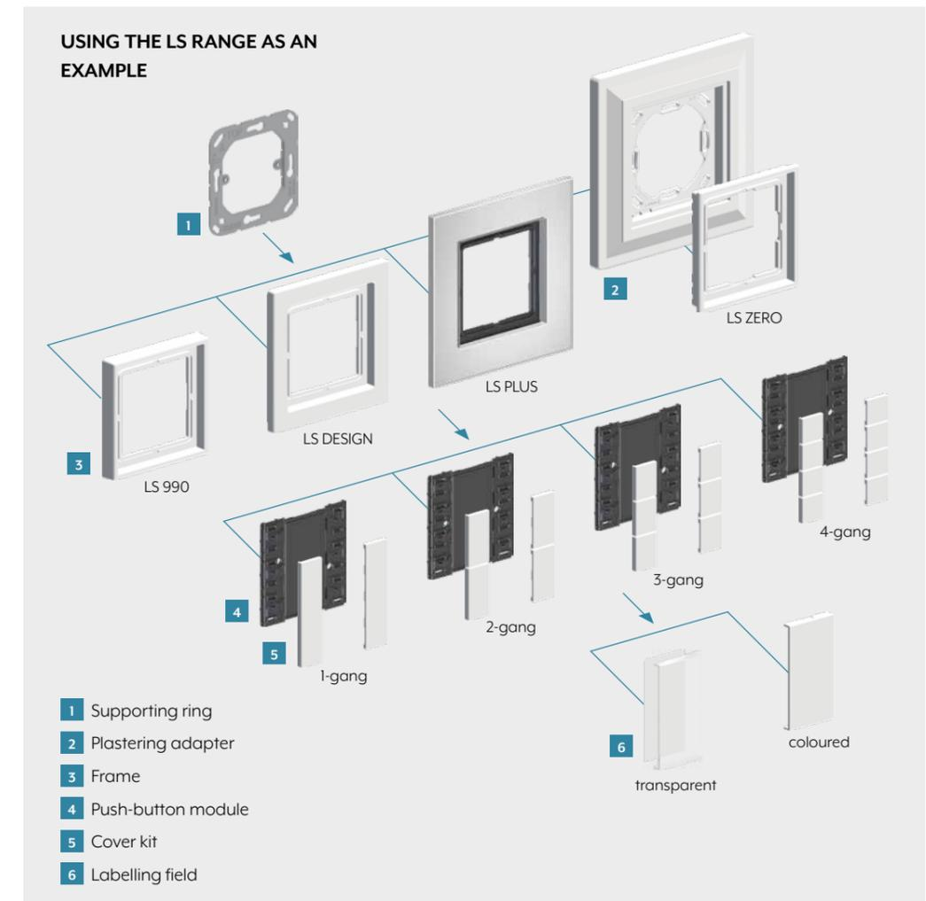
The 1, 2, 3 and 4-gang F 50 modules are available in the JUNG design alongside the corresponding 1 to 4-gang cover kits. The transparent or coloured labelling field is optionally added to this. The design frames of the various ranges round off the concept.
